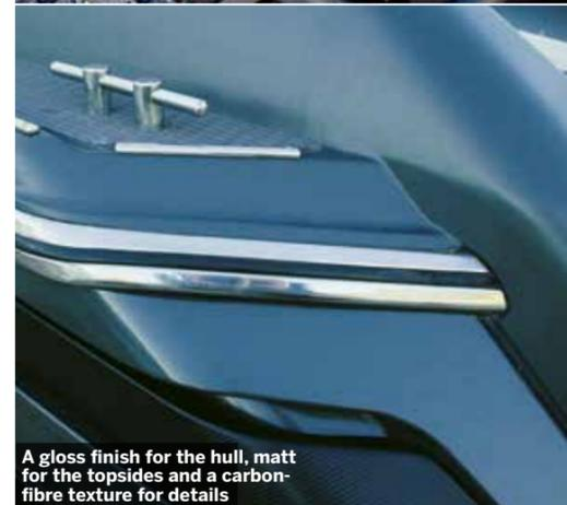
A gloss finish for the hull, matt for the topsides and a carbon-fibre texture for details
