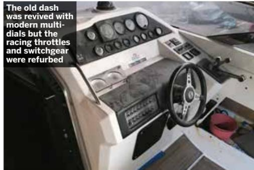
The old dash was revived with modern multi-dials but the racing throttles and switchgear were refurbished
