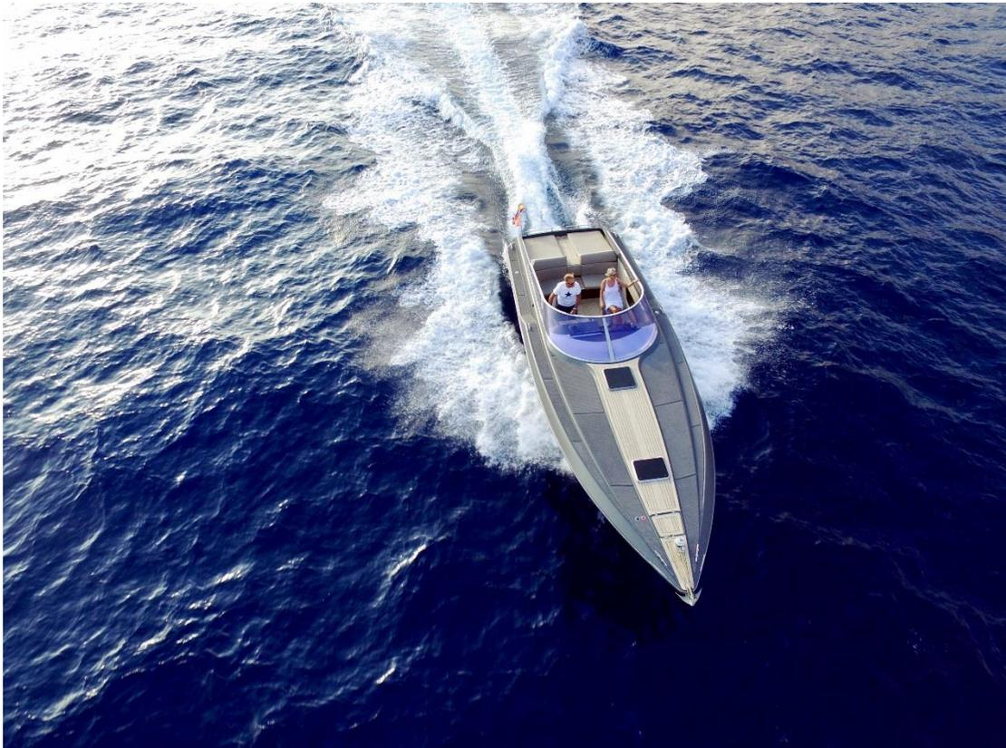
The removal of the radar arch has contributed significantly to creating the sleek, purposeful profile. This has been further emphasised by continuing the rake of the screen line to the aft, with a stainless steel handrail, echoed in new rails to the stern.
